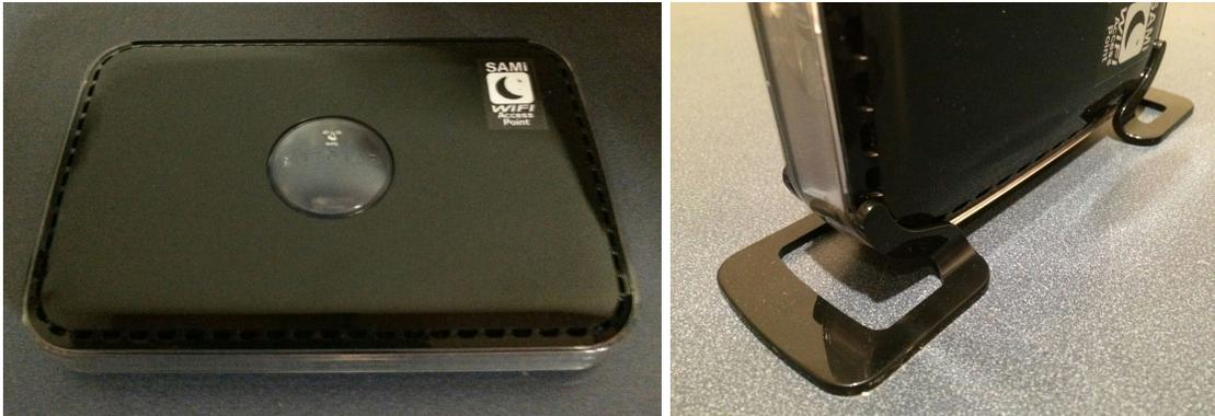
Unpack and **plug in the WiFi Router.** Ideally, pick at a location about halfway between where the camera will be mounted and where you plan on using the iPad. Best location is up high. Use the supplied clip-on stands if you want the router to stand up. Make sure the router is turned on; the switch is in the back.
